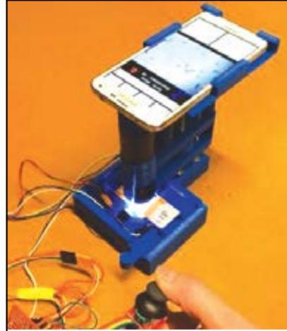
The LudusScope is an interactive smartphone microscope that can be made entirely out of 3D printed or commonly available materials and is easily assembled by middle school or high school students. Developed by Stanford bioengineer Ingmar Riedel-Kruse, it allows students to interact directly with light-sensitive microorganisms called Euglena. 3D printing plans are open source, as is the software for the interactive smartphone tools.
