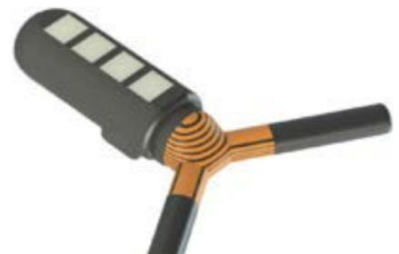
all of the various components carried by the capsules, and to build the capsule from alternating layers of stiff and flexible polymers, which helps it to withstand the acidic environment of the stomach.
